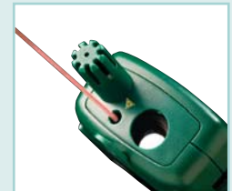
Patented IR thermometer design locates cold spots on walls, which identifies surfaces subject to condensation (direct differential display of IR - DP)
